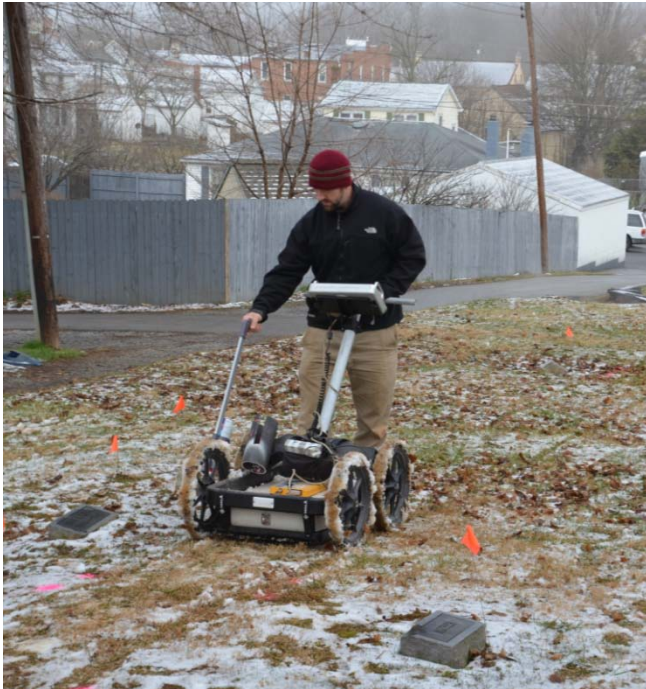
Figure 38. GPR being conducted in the cemetery. A light snow occurred during the work, but did not affect results.
