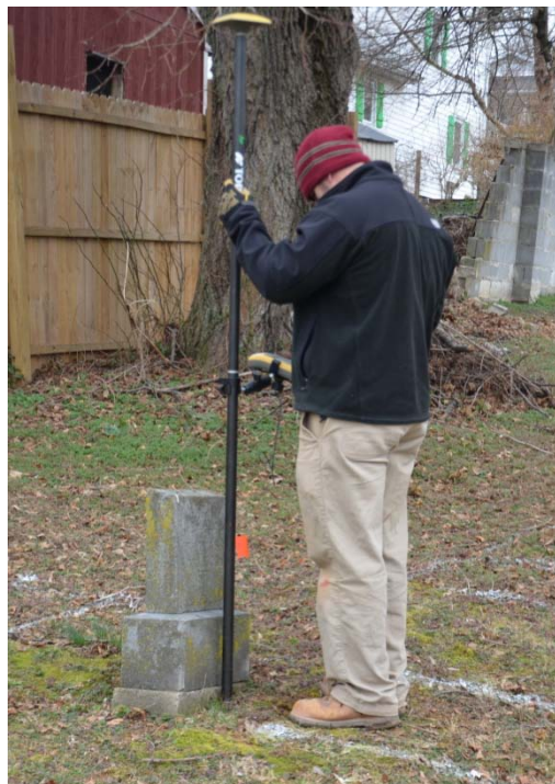
Figure 39. Mapping the cemetery using a sub-meter GPS system.
